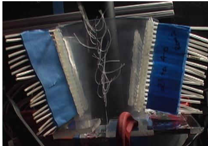
Figure 4.24 : Tufts on diffuser 2 with dump gap ratio of \infty
