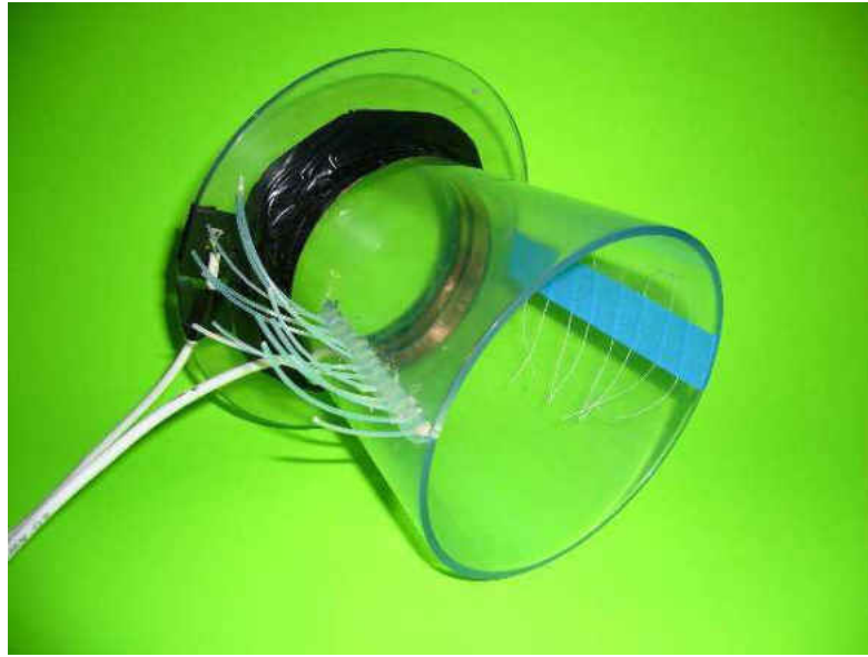
Figure 3.7: DBD plasma actuator arranged on diffuser model
