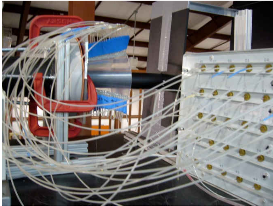
Figure 3.6: Scanivalve setup attached to static pressure ports on diffuser 2
